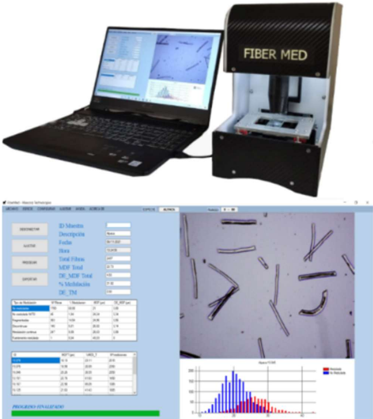
Figure 1. Top: Intelligent electronic medullator of animal fibers (Fiber Med) that was used for the analysis of white alpaca fibers. Down: Graphical user interface (GUI) of the device.
